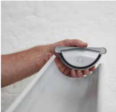
Stop ends These ends are self-sealing with an EPDM tube. They are fully reversible, i.e. same unit fits on both left and right end of a gutter. And they are easily mounted with just a single, firm knock.
