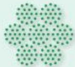
Rope 6 × 19 + WC for Webnet rope Ø 3.0 mm
