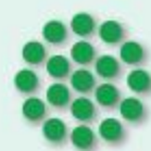
Stranded wire 1 × 19 for Webnet stranded wire Ø 1.0 mm, 1.5 mm, 2.0 mm, and 3.0 mm
